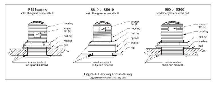
**Metal hull**—Use the spacer if there are not enough threads to tighten the hull nut against the hull.
