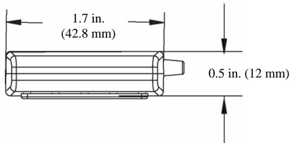
**Figure 2. GPS 20x Side View**
