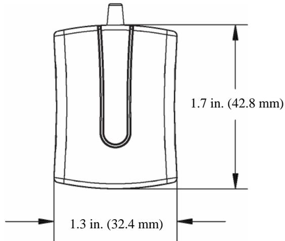
**Figure 1. GPS 20x Top Case Dimensions**
